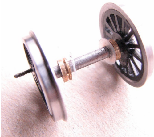
Assembled wheels for the non-g geared axles. Note from left to right on the axle; 1mm & 0.5mm spacers, Heljan plastic or Peco fibre washer, plastic or fibre washer and 1mm & 1.5mm spacers.
