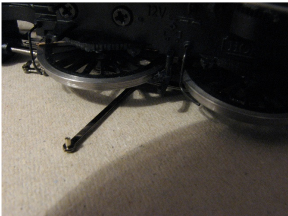
Rod with rivet in place through hole.
