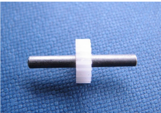
Assembled axle and Heljan gear.
