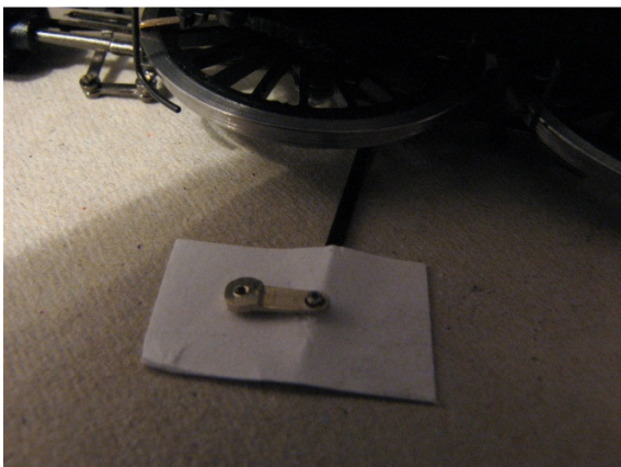
Paper placed over rivet with crank placed on top ready to solder.
