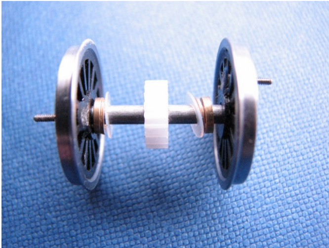
Driven axle assembled with spacers plus plastic washers.
